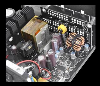
High Amperage Single +12V Rail & DC to DC Design
