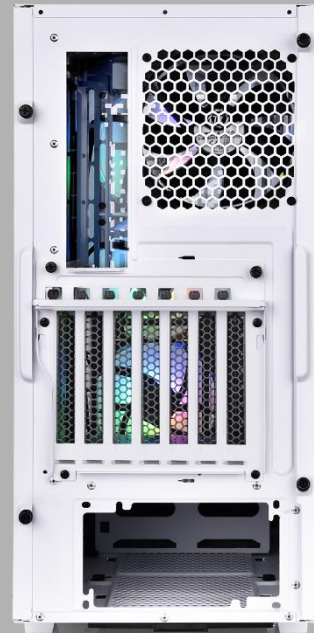
Vertical VGA installation
